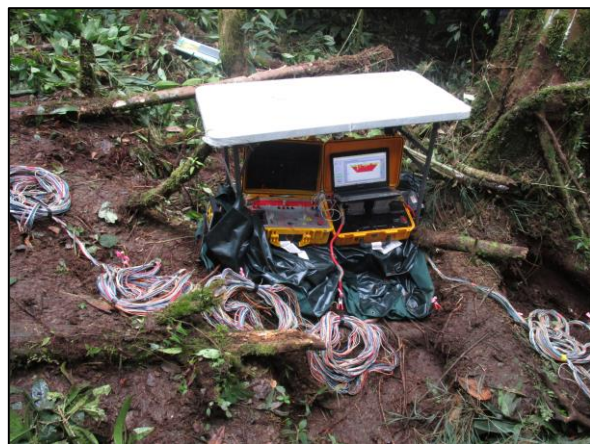
A ground search being conducted in the Colombian Jungle, using geophysics (ERT) and an explosive detection dog in Colombia (Source: Carlos Molina 2018).
