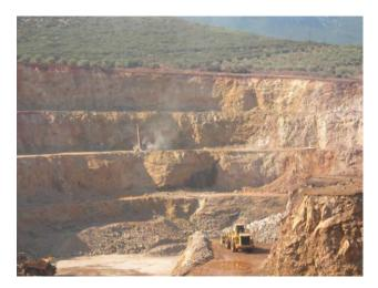
Figure 22: Modern open-pit mining of iron-nickel laterite employing sophisticated blasting technology, large haulage trucks and Doppler radar systems to monitor slope stability, Agios Ioannis mines at Neo Kokkino, Larymna, Greece. Photo: A. Demetriades
