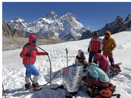
IGCP 672: Students practicing using Stream Drill to install an ablation stake at Changri Nup Glacier in the Everest region of Nepal. © Dibas Shrestha and Guillem Vincent
